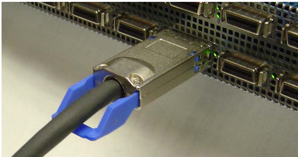
Figure 3-10: Fully Installed IB Cable with Pull Connector
